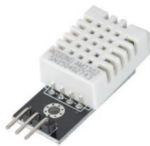
Fig. 2. DHT22 temperature and humidity sensor
